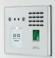
MB560-VL is a multi-biometric identification terminal featuring ZKTeco's innovative Visible Light Facial Recognition technology.
