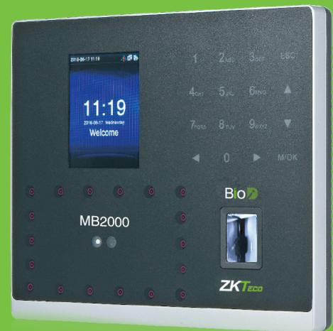
MB2000 is Time & Attendance and Access Control Terminal to be associated with BioID fingerprint reader, face recognition and RFID card functions. With the new BioID fingerprint reader, the operation remains stable under strong light source and high preciseness of verification of wet and rough fingers. With latest facial algorithm and the innovation features, MB2000 is bringing you the whole new experience.
